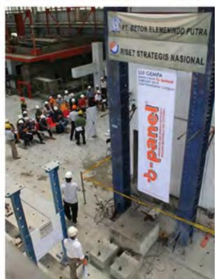
b-panel® earthquake test at PUSLITBANGKIM Cileunyi (Indonesia earthquake zone-6 simulation)
